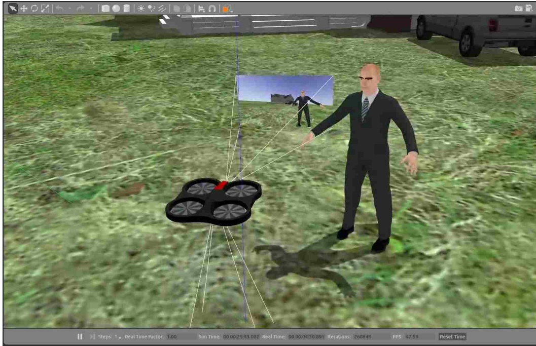
Figure 3.3: Simulated AR.Drone model with video streaming from the frontal camera along with readings from its sensors in real-time inside a 3D custom environment generated via the Gazebo simulator.
